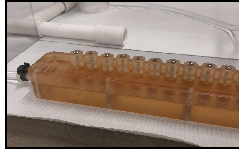
Modified Robins Device for biofilm formation
