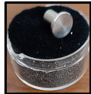
Stainless steel coupon (surface for biofilm)
