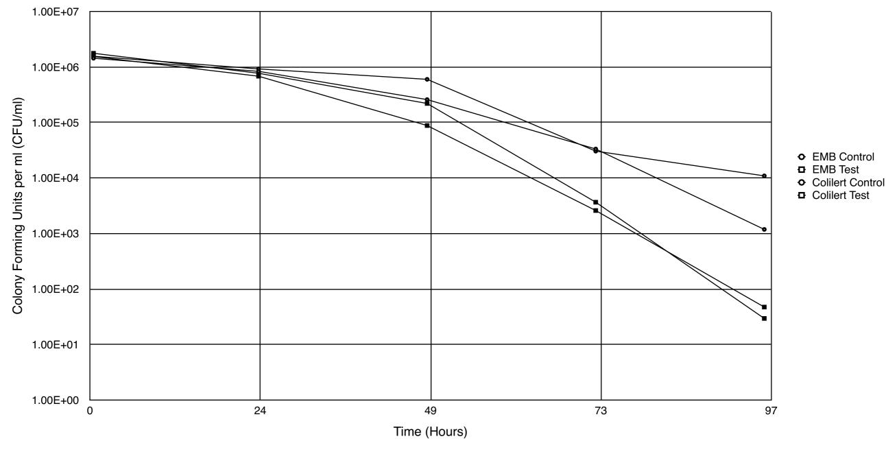
\*Graph shows results from Phase 1 of the academic research using two different testing methods EMB & Colilert Highlighted in blue are the two different testing methods test results of the drop in unit. In Yellow is the control test with out the drop in.
