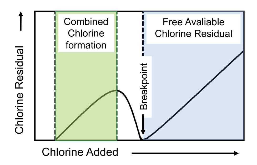
When chlorine is added to contaminated water combined chlorine is formed, which adds to the chlorine demand of the system. As more chlorine is added the combined chlorine is oxidized resulting in the "**breakpoint**" as the combined chlorine is consumed. After the "breakpoint" additional chlorine is as a free chlorine residual and which can oxidize any additional contaminants
